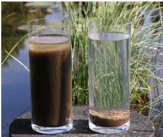
Figure 2: Sludge settleability: activated sludge (left side cylinder) vs. Nereda® aerobic granular sludge (right side cylinder)
