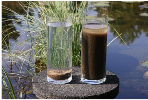
Figure 1. Settling Properties of the Aerobic Granular Biomass (left) compared to Activated Sludge (right)
