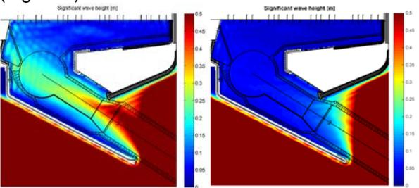
Figure 8 Significant wave height in the port for all frequencies (close up of Figure 6, different scale)
