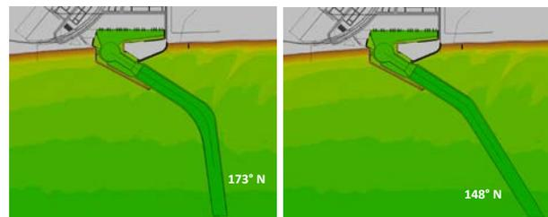
Figure 5 Two considered orientations of the entrance channel
