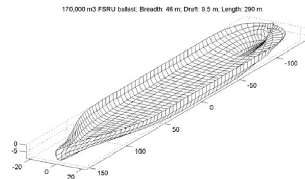
Figure 3 3D mesh of the ship used for time-domain diffraction analysis
