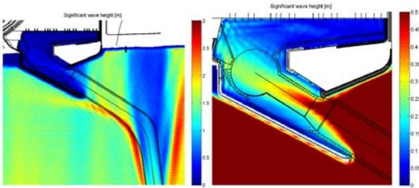
Figure 7 Wave trapping on the side of the entrance channel for 180°N wave direction
