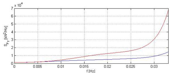
Figure 11 Surge and sway wave force spectra on general cargo vessel (low frequency range)
