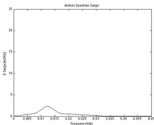
Figure 20 Surge motion response spectrum, with ShoreTension® (2<sup>nd</sup> measurement)
