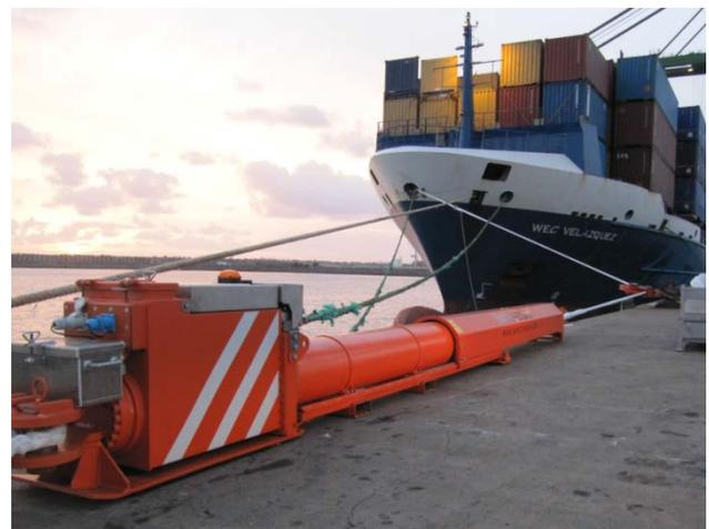
Figure 14 ShoreTension® cylinder added to the mooring layout as an additional breast line
