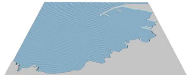
Figure 1 Area required for the simulation of the wave penetration of the port basin on the top right to ensure that the free long waves reflected from the coast are captured
