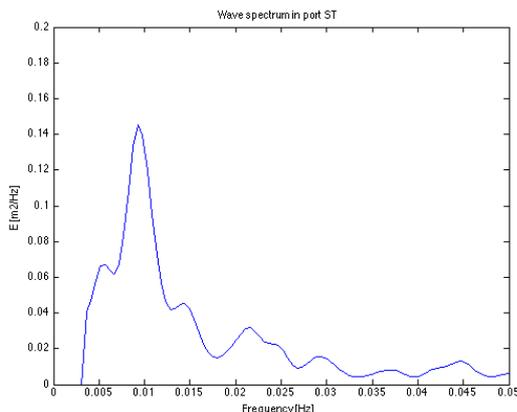
Figure 15 Measured spectrum water elevation in the port basin during the 1<sup>st</sup> measurement
