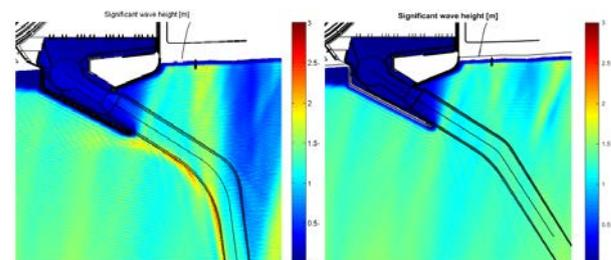
Figure 6 Significant wave height in entire domain for all frequencies
