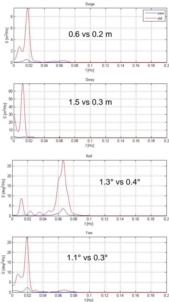
Figure 12 Surge, sway, roll and yaw response spectra, including significant motion amplitude, for the general cargo vessel
