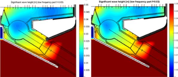
Figure 9 Significant wave height in the port, only low frequency part (<0.03 Hz)
