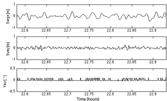
Figure 18 Time-series measured surge, sway and yaw motion, with ShoreTension® (2<sup>nd</sup> measurement; x-axis in hours)
