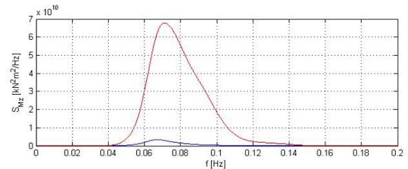
Figure 10 Surge, sway, roll and yaw wave force spectra on general cargo vessel
