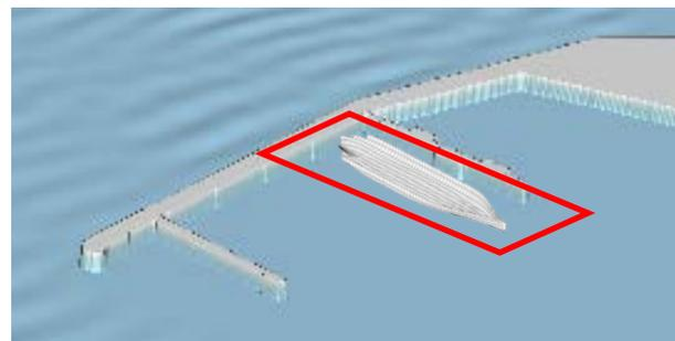
Figure 2 Output area wave penetration model around the ship required for time-domain diffraction analysis
