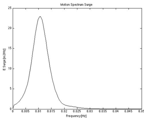
Figure 19 Surge motion response spectrum, without ShoreTension® (1<sup>st</sup> measurement)
