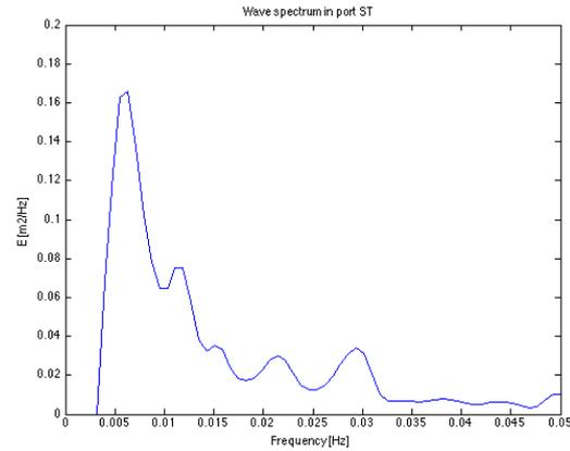
Figure 16 Measured spectrum water elevation in the port basin during the 2<sup>nd</sup> measurement
