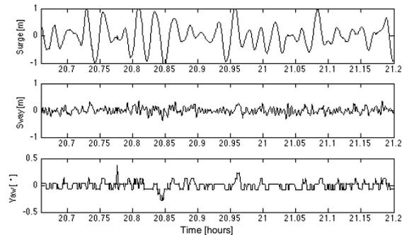
Figure 17 Time-series measured surge, sway and yaw motion, without ShoreTension® (1<sup>st</sup> measurement; x-axis in hours)
