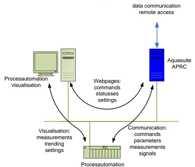
Crystalactor Controller generates operator friendly webpages for visualization of status, settings, measurements, calculations and trends. These pages can be easily accessed on any computer on the network and/or integrated into the standard visualization system.
