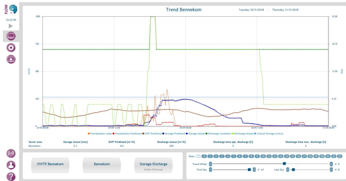
**Figure 5: Example of peak flow reduction after a rainfall event at WwTP Bennekom using predictive control with rainfall forecast for the event of 29 May 2018**
