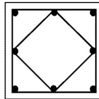
**Figure 12** Example of additional concrete column rebar for earthquake loading according to EN 1998-1
