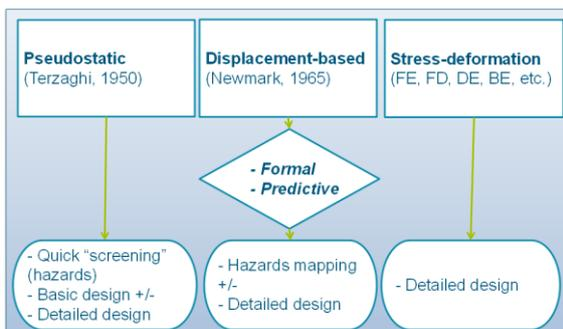
Figure 4 Approaches calculate co-seismic slope stability
