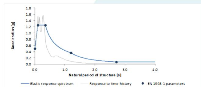
Figure 7: Examples of elastic response spectra
