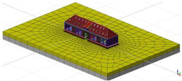
**Figure 10** Finite element model of a building with soil for non-linear time history analysis
