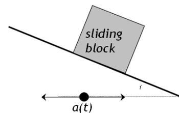
Figure 5 Seismic destabilizing force acting on the sliding block
