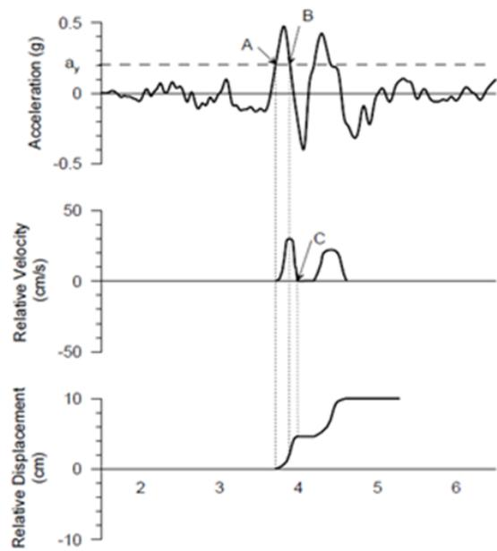
Figure 6 Newmark analysis principle
