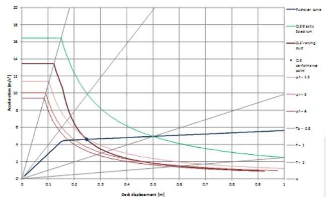
Figure 9 Example of push-over analysis results
