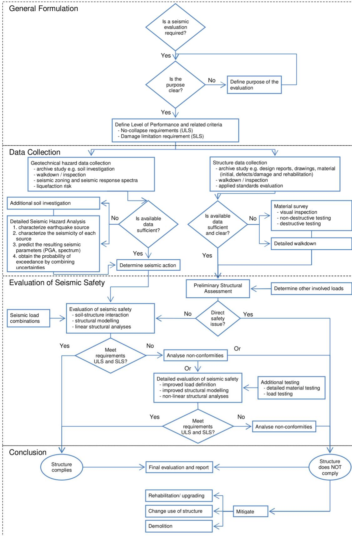
Figure 2: flow chart for a quickscan of risks related to earthquake loading
