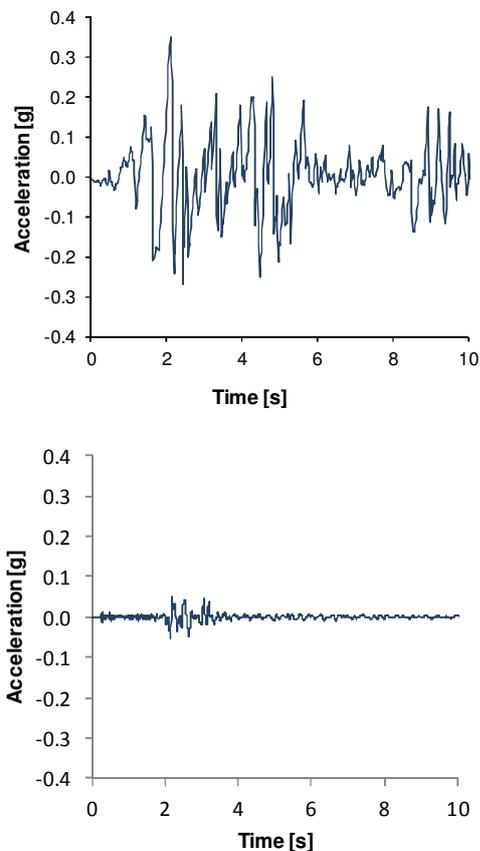
Figure 3 : example of recorded tectonic earthquake time-history (El Centro, Mexico 1940, top figure) and induced earthquake time-history (Westeremden, the Netherlands 2012 )
