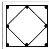
**Figure 6 : example of additional concrete column rebar for earthquake loading according to EN 1998-1**
