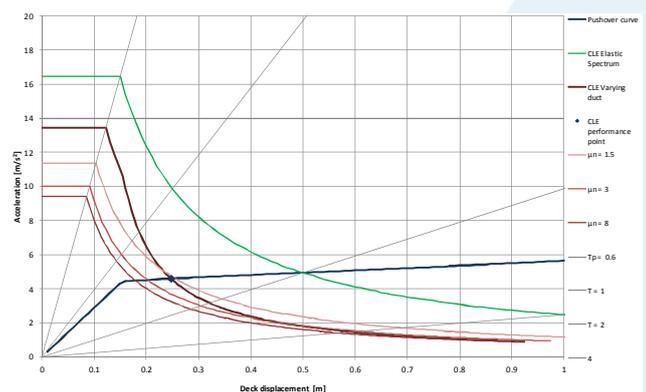
Figure 4 example of push-over analysis results
