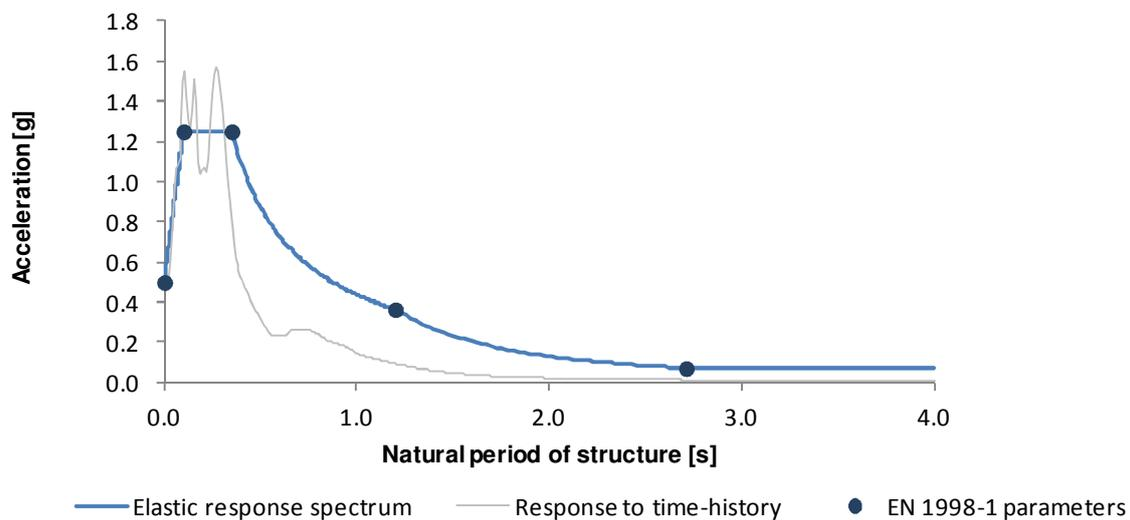
Figure 1: example of 5% damped horizontal elastic response spectrum based on the formulation in EN 1998-1 and example of the 5% damped elastic response to a single time-history
