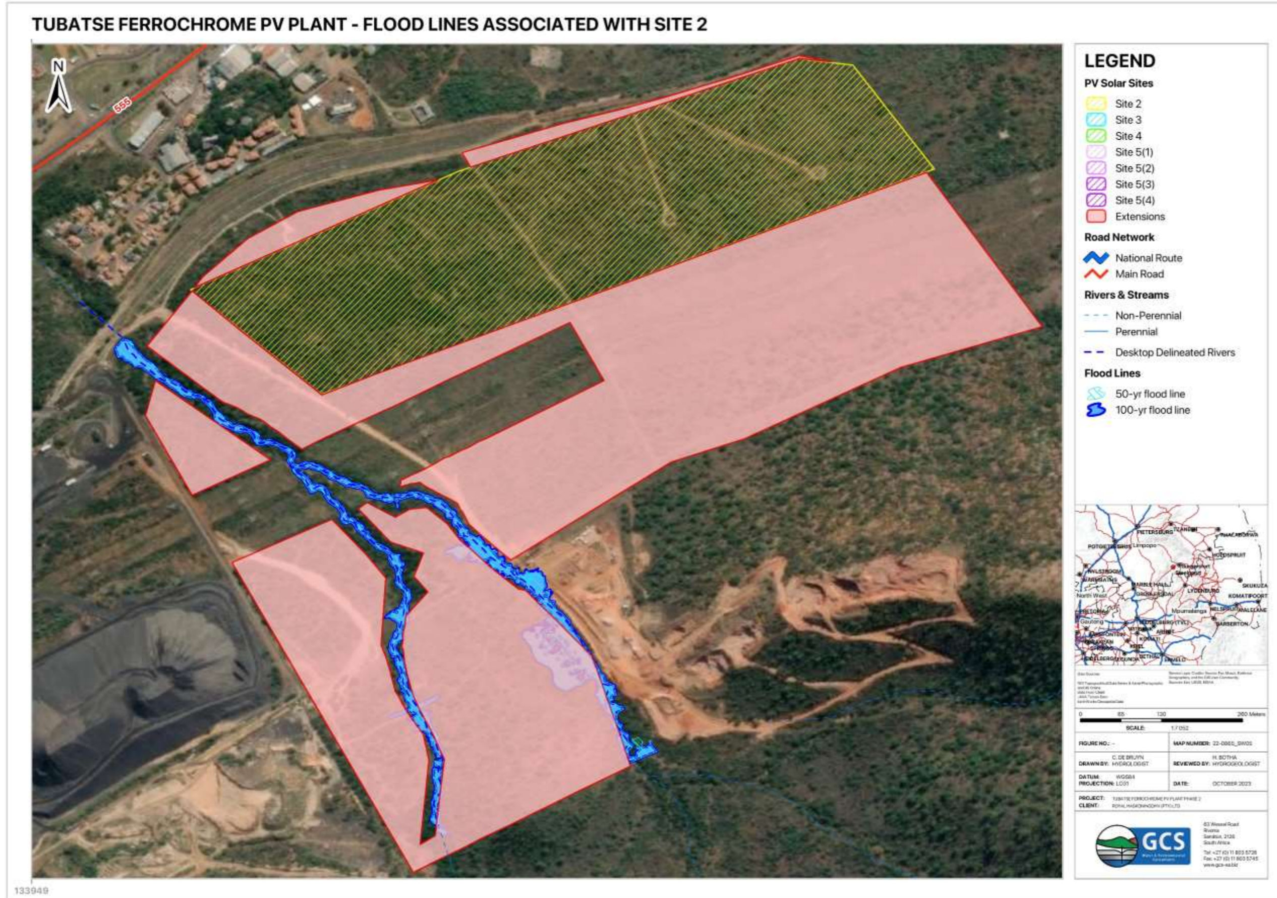
Figure 5-2: Simulated flood lines for the tributary flowing adjacent to site 2 and expansion sites
