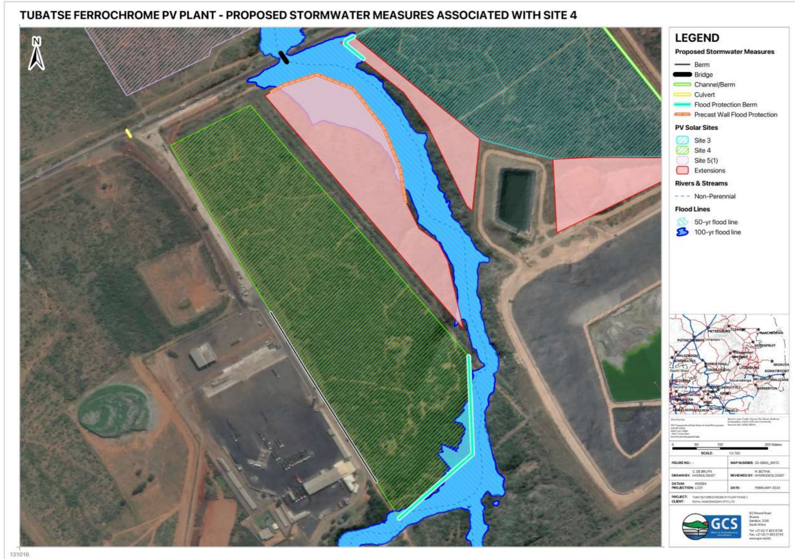
Figure 6-15: Proposed stormwater infrastructure for Site 4
